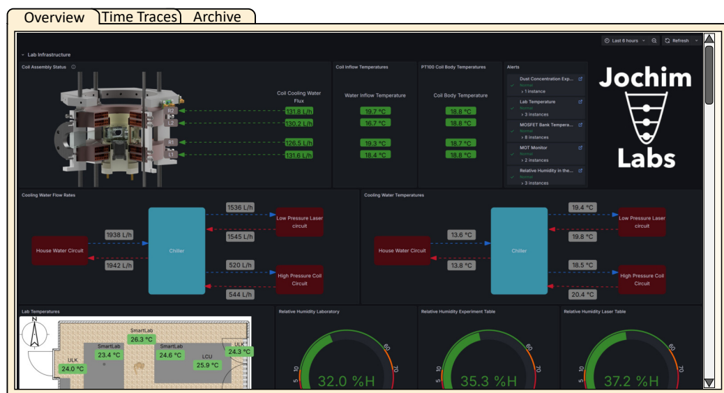
Figure 4.21: Example snippet of HQA-ONE’s Grafana homescreen for operations status and metric monitoring. Visible in this snippet are performance representations of the water cooling system, alert status, and environmental data of the laboratory from the different air conditioning units and individual custom sensors. The tabs of the sketched window illustrate different functionalities covered by SmartLab as well, including time traces for all measured metrics and a long-term data archive for these readings.
