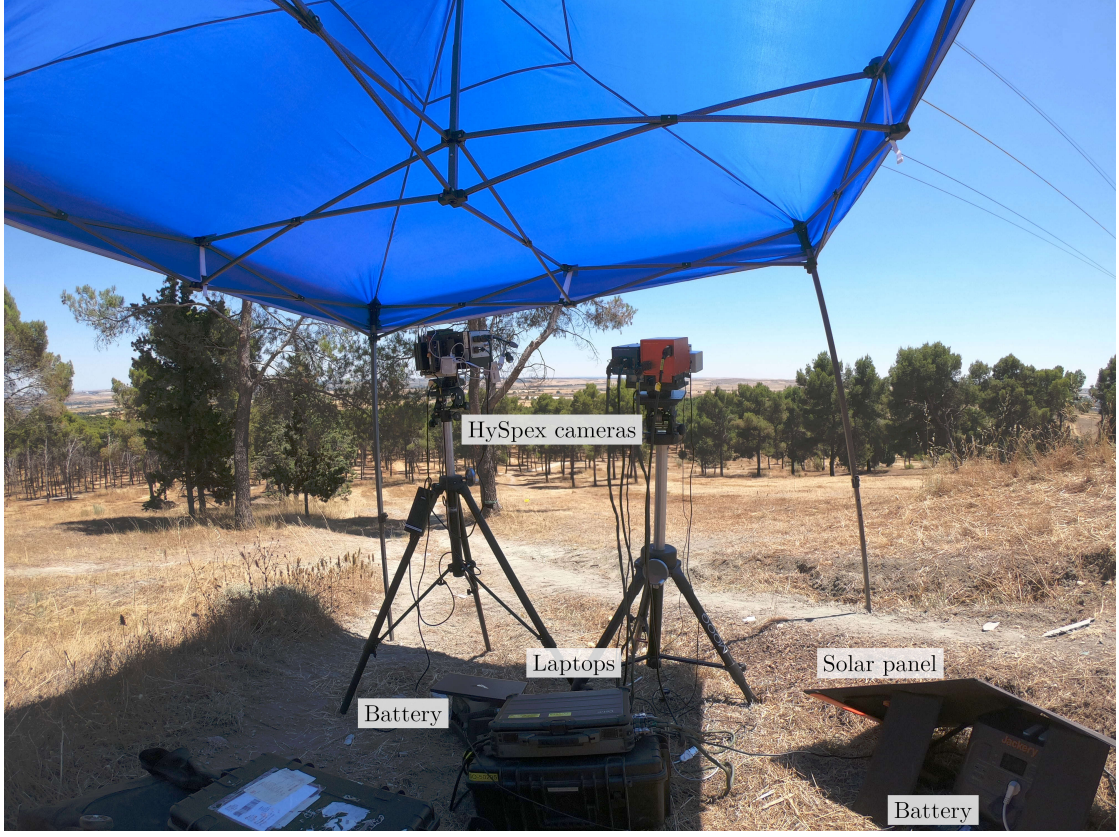
Fig. 3.1. The measurement setup on July 4, 2024, at the Pinto landfill. The black camera on the left tripod is the HySpex Mjolnir S-620. The blue camera on the right tripod is the HySpex VNIR-1800 and the red camera on the right tripod is the HySpex SWIR-384. The cameras and rotation stages are controlled by two laptops, and all devices are powered by two battery packs and a solar panel.
