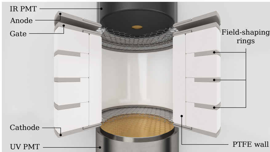
Figure 8.7.: Schematic drawing of the HeXe time projection chamber (TPC) with the IR-sensitive PMT at the top. During operation, LXe is filled in the cylinder with a liquid level maintained between anode and gate (not shown here). Reproduced from [Paper VI].
