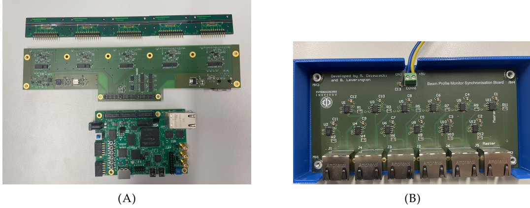
FIGURE 4.3: Electronics of the SciFi-BPM. (A) One BPM plane, from top to bottom: five photodiode arrays, the sensor readout board (hosting five ADCs), and the FPGA board. (B) Synchronization board.
