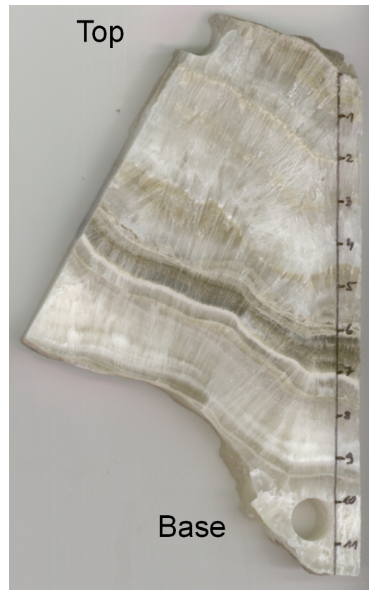
Fig. 4.7: Slice of flowstone SPA 59 . The black scale bar indicates the growth axis. Numbers give the distance from the top in cm. Note the multiple hiatuses representing periods of growth interruptions.
