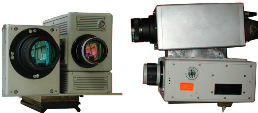
Figure 6.1: Infrared stereo camera setup: front (left) and top (right) views.
