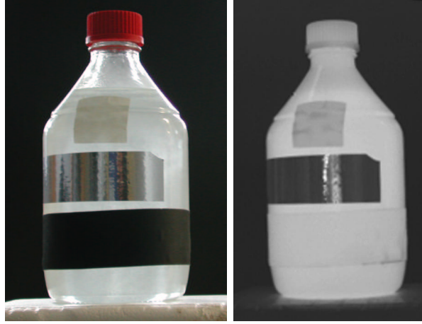
Figure 2.11: Effect of emissivity: The left image shows a color photograph of a bottle with a white sticker, aluminum coated tape, and black duct tape. The bottle is filled with warm water. In the infrared image on the right the white sticker and the aluminum tape appear darker because of their lower emissivity compared to the black tape and the bottle glass.
