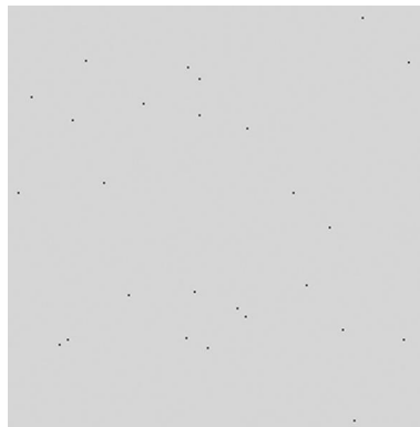
Figure 7.5: Binary mask of the pixels of the Amber Radiance detector which, despite the on-board correction, were identified as bad pixels by the distance-from-fit criterion. Bad pixels are displayed in black, good pixels are displayed in grey.
