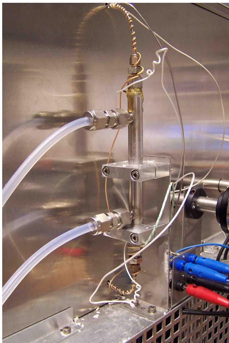
**Figure 5.8 :** *The  $H_2O$  focus unit of the analytical system. Shown are the teflon lines for the evaporated liquid nitrogen, and the coiled heating wires.*
