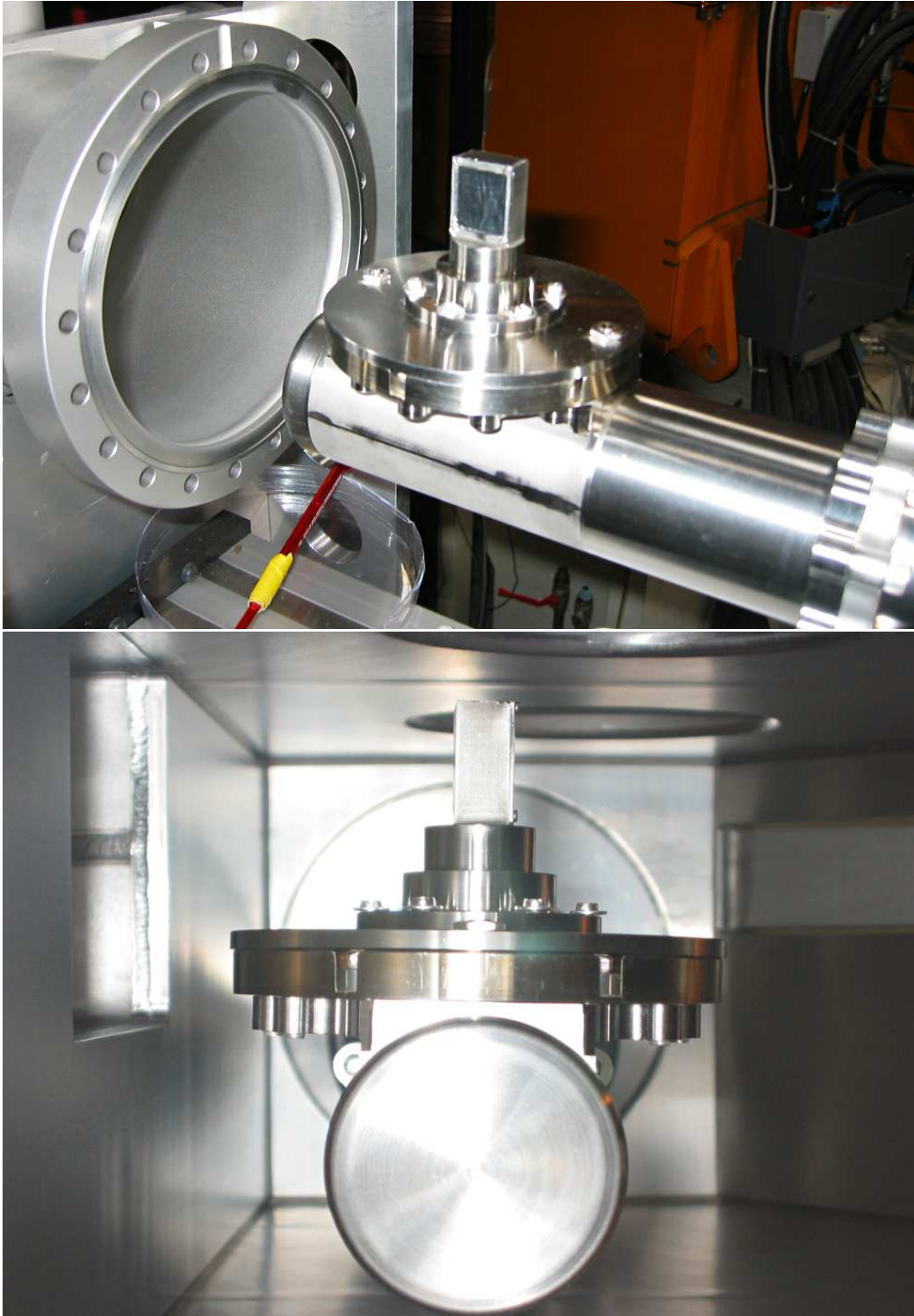
Fig. 3.4: Upper: Head of the detector before installation into the vacuum system. Lower: The MIDAS detector inside of the dipole chamber. On the left Product fragments enter from the right. The stored ion beam passes above the cylindrical support tube into the ongoing TSR beamline.
