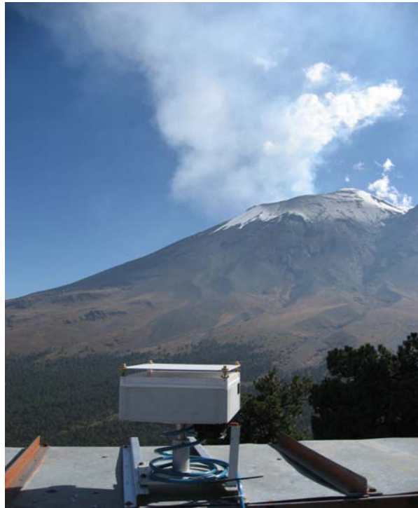
Fig. 5.16 – NOVAC mark II instrument installed at the site tlamacas_hd, approximately 5 km north of Popocatepetl Volcano (Mexico). The instrument is located on the premises of a radio-antenna station at 4030 m a.s.l., therefore power is supplied by land line. The rest of the installation (battery, charger, timer, radio modem) are located in a box below the metal cable shaft on which the instrument is mounted, and are connected via the blue cable shown in the image. The instrument is equipped with a sun shield to reduce heating by solar radiation.
