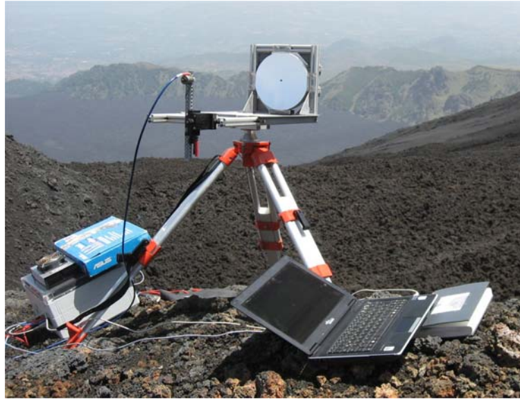
Fig. 3.46 – Miniature Active Long Path DOAS designed for application in remote environments. The blue fiber bundle is positioned in the focal point of a 20 cm diameter spherical mirror, thus emitting nearly-parallel light. After being reflected back to the telescope by an array of retro reflectors, the central fiber in the bundle couples the incident radiation into the spectrometer. Here, an Ocean Optics QE65000 spectrometer was applied, located in a temperature stabilized housing (bottom left of the image). The measurements are controlled by a laptop computer.
