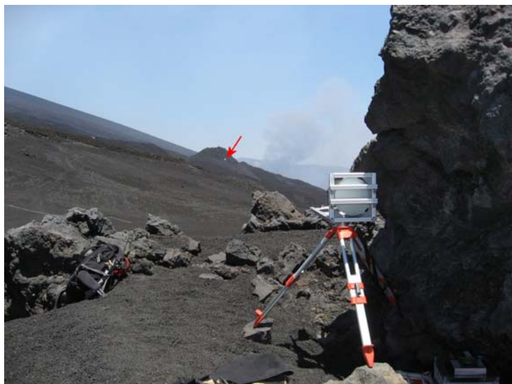
Fig. 7.17 – LP-DOAS setup at site 4, about 2 km downwind of the summit craters (see Fig. 7.15) on July 10, 2008. The red arrow again indicates the reflector position. Extreme wind speeds of approximately 20 m/s pushed the volcanic plume down along the eastern flank of the mountain, thus making downwind measurements with the LP-DOAS possible. The instrument was placed as close as possible to a solid rock ledge to shield the telescope from dust and rocks picked up by the strong winds. The explosion seen in the background originates from a newly formed vent. Explosions of increasing intensity at this vent forced the measurements conducted the previous day at site 3 to be aborted and scientists to be rapidly evacuated.
