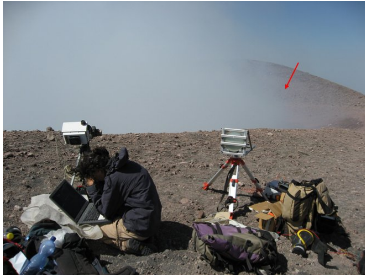
Fig. 7.16 – Image of the LP-DOAS measurements (right) conducted at the NE crater of Mt. Etna (site 2 in Fig. 7.15). The red arrow indicates the position of the retro reflector array. Supplementary MAX-DOAS measurements (left) were conducted simultaneously by Nicole Bobrowski.
