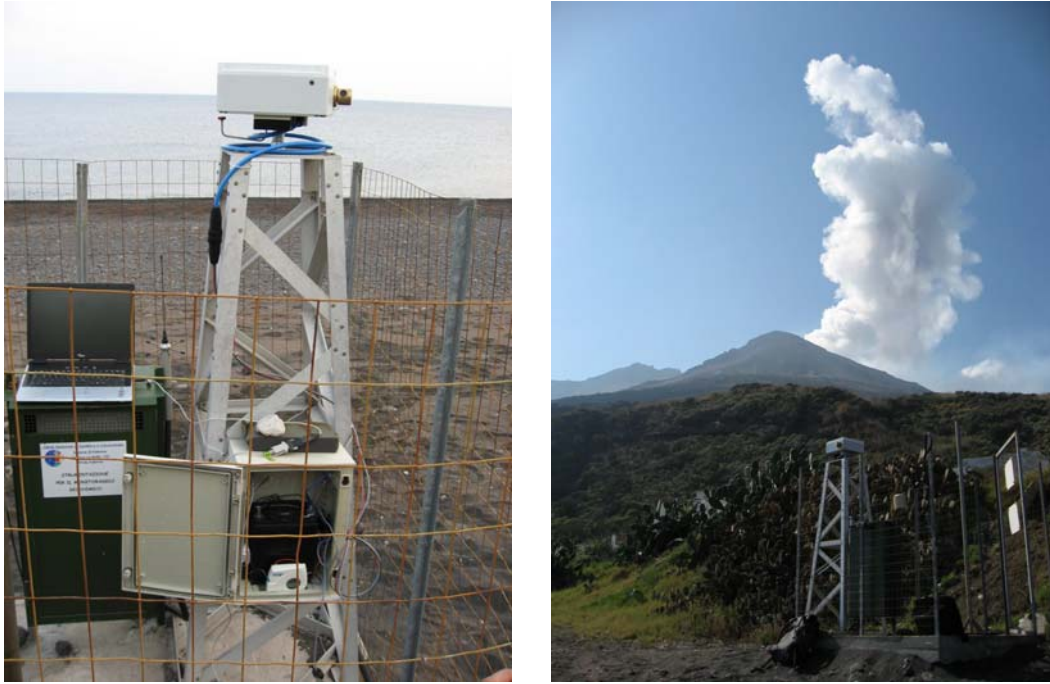
Fig. 5.5 – Both images show the NOVA test installation at Pozzo Saibbo, Stromboli. The NOVA mark II instrument is installed on an approx. 2 m aluminum tower on the beach just southwest of the ferry landing. Power is supplied by a 12 V land line. A 40 Ah battery in the electric installation box at the base of the tower is used as a buffer in case of short term power outages. A timer switches the instrument off at night. A data link has not yet been established, so measurement data needs to be downloaded using a laptop computer.
