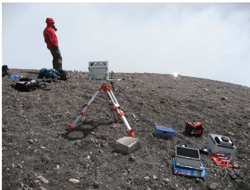
Fig. 3.8 – Active Long Path DOAS measurements conducted at Mt. Etna on July 15 of 2008. Here, a light path of only 2 \times 20 m was used (site 5 in Fig. 7.15), as SO 2 mixing ratios in the order of 100 ppb regularly caused virtually complete absorption of radiation between 290 and 310 nm (see Fig. 3.23).
