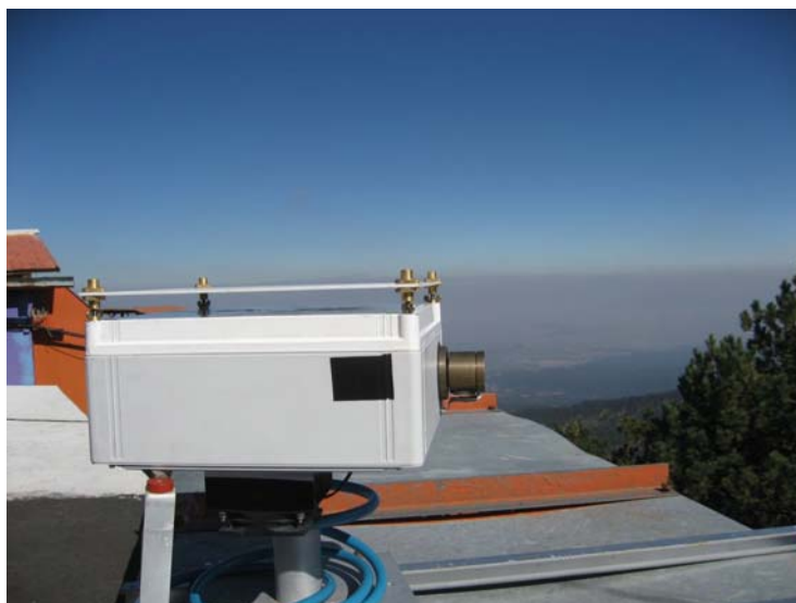
Fig. 5.21 – Viewing direction of the NOVAC mark II instrument during measurements of urban pollution and biomass burning in the Puebla Valley, 130 km southeast of Mexico City. The boundary layer is clearly distinguishable as an area of brown haze.
