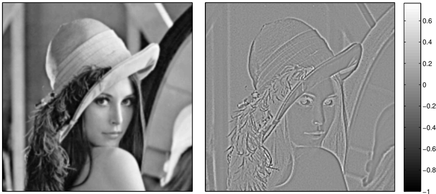
Figure 5.13: Illustration of the curvature measure (5.17) for the "Lena" image.
