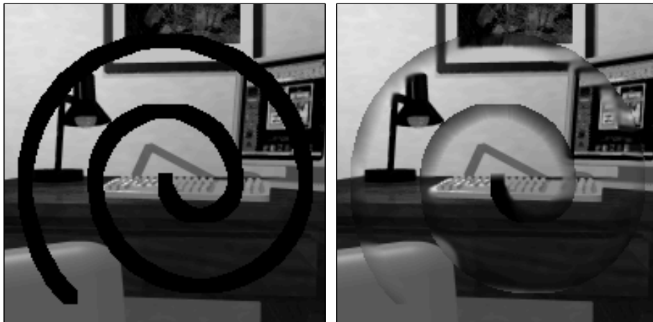
Figure 6.6: Image reconstruction with a divergent transport vector field. Left: "Office" frame with inpaint region (black spiral). Right: Inpainting result. If the image information is transported with a divergence velocity field, the image intensity decreases within the inpaint region due to the deformation of the image structure.
