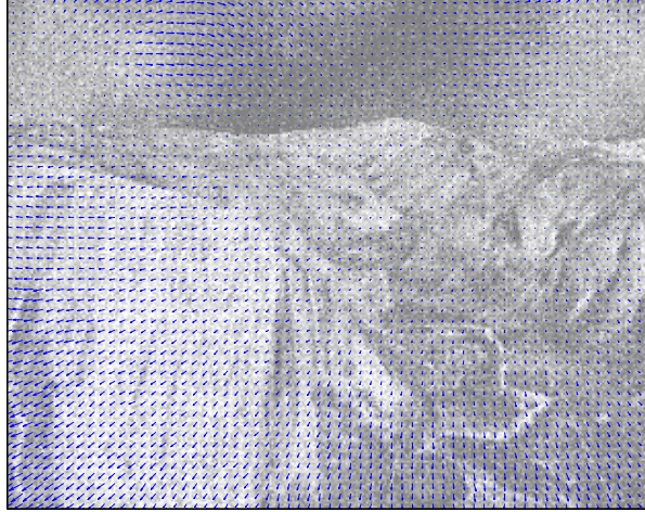
Figure 4.9: Temporal regularisation. We added Gaussian noise with standard derivation \sigma = 40 to the "Yosemite" sequence. The shown optical flow field is obtained by the control based optical flow approach (4.3 - 4.4) (parameters: \alpha = 0.05 and \beta = 0.000003 ).
