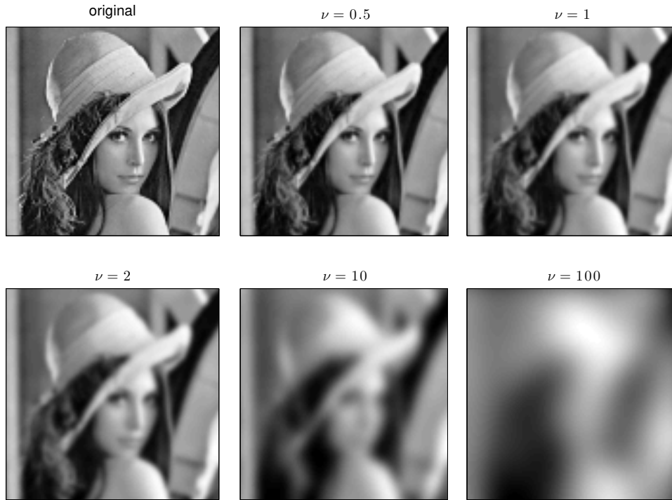
Figure 7.2: Diffusion process demonstrated at the well-known "Lena" image. The first image in the first row shows the original "Lena" image. The second image shows the computational result for the diffusion equation with a kinematic viscosity coefficient \nu = 0.5 . The following images are computed with viscosity values \nu = 1 , \nu = 2 , \nu = 10 and \nu = 100 . For further increasing values of \nu all pixel intensity values of the image converge to the mean grey value of the image.
