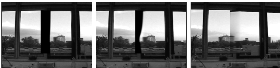
Figure 6.12: The "Mannheim office" sequence with a large inpaint region (size: 30x150 pixels). Left: Single frame of the "Mannheim office" sequence along with the inpaint region in the middle of the image. Middle: Video inpainting result for frame 4 of the sequence. Right: Inpaint result for the last frame.
