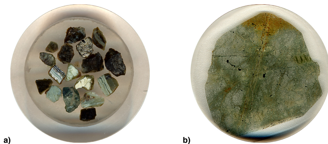
Fig. 2.2: Examples of 1-inch round samples: a) micro-section FIH4-2, b) thin-section A012R01W(3-5), partly serpentinitized areas appear green, entirely serpentinitized and brucite-bearing areas appear brownish to yellow.
