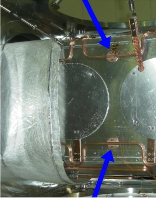
Figure 3.10: Photo of the 80 K thermal shields with water cooling lines (contact points with the shield are marked with arrows) and multilayer insulation (on the left) visible. A braided copper wire used to thermally anchor one of the chamber suspension wires is visible in the upper right corner. Two access ports to the enclosed 40 K shields and vacuum chambers can also be seen.
