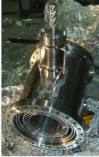
Figure 3.19: Photo of the bake-able, charcoal-based, UHV cryopump.
