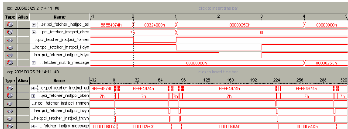
Figure III-16: Asynchronous reception of feedback messages at the scheduler. Five transactions can be distinguished in the lower trace. Each one represents the transfer of a feedback message originating from a different computing node.
