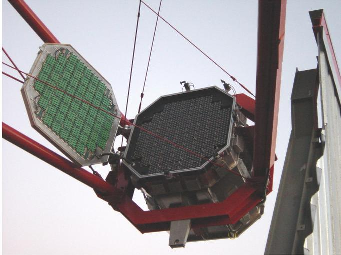
Figure 2.10: The imaging camera of a H.E.S.S. telescope.
