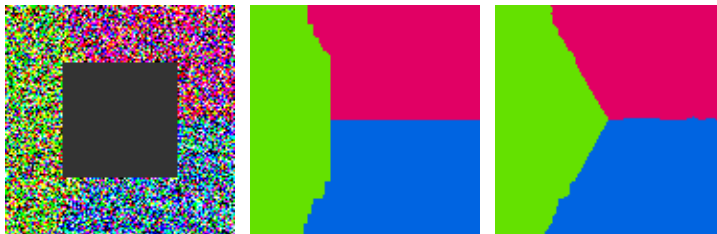
Figure 3: Effect of the discretization on an inpainting problem. Left to right: Input image with unknown black region; graph-based method using pairwise potentials ( \alpha - \beta -swap code from [SZS + 06]); proposed method using higher order potentials. Due to the introduced anisotropy, the graph-based method shows a bias towards axis-parallel edges.
