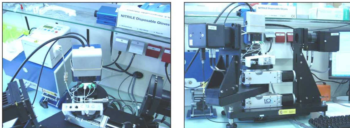
Figure 6.11: Images of the combined QCM-D/ellipsometry set-up.
