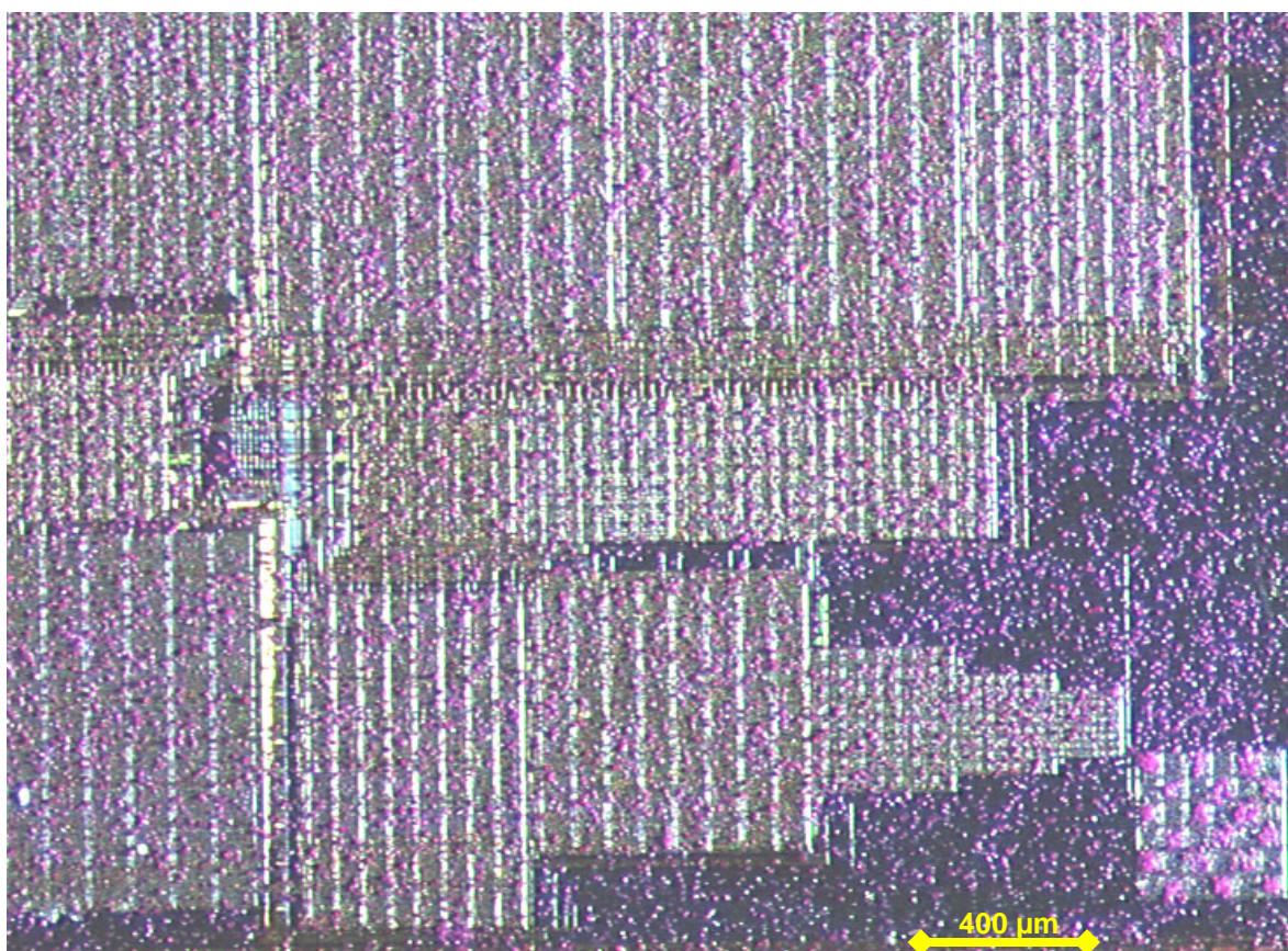
Fig. 6.28: Example of particle deposition on a Peptidchip 3.1 with 50% PEGMA, 50% MMA layer (thickness ca. 50-100 nm). Selective particle deposition failed, except for the pixels with passivation openings (lower right).
