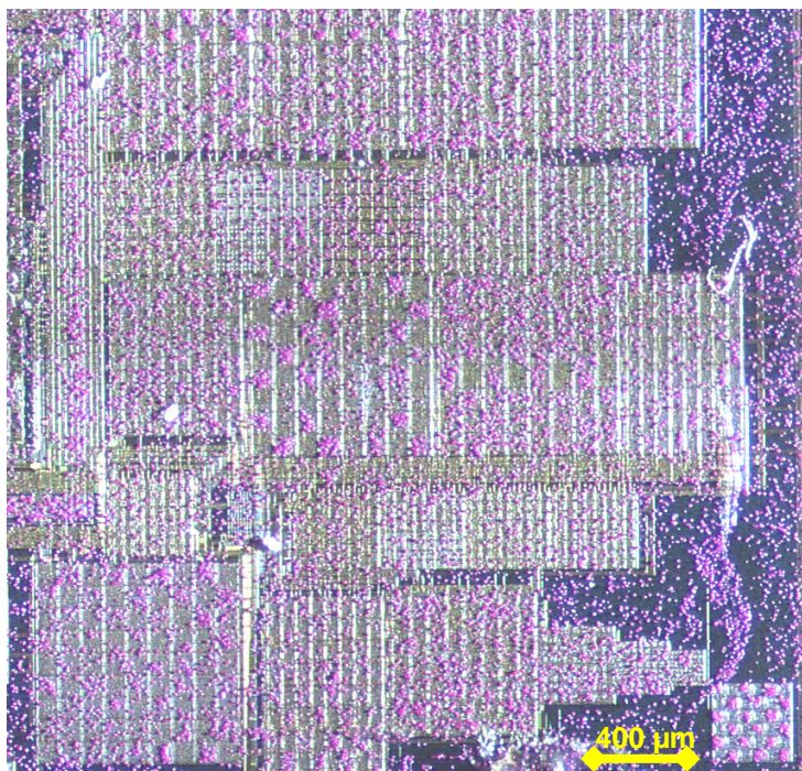
Fig. 6.27: Example of particle deposition on a Peptidchip 3.1 with thin PEGMA layer ( \approx 35 \mu\text{m} ). Selective particle deposition is successful only on some pixel matrices. Deposition was performed without chip covering installed. Stitched microscope images.
