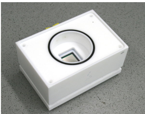
Fig. 5.20: Peptidchip 5 on PCB with covering, installed into the synthesis chamber. The silvery area in the center is the pixel area of the chip.
