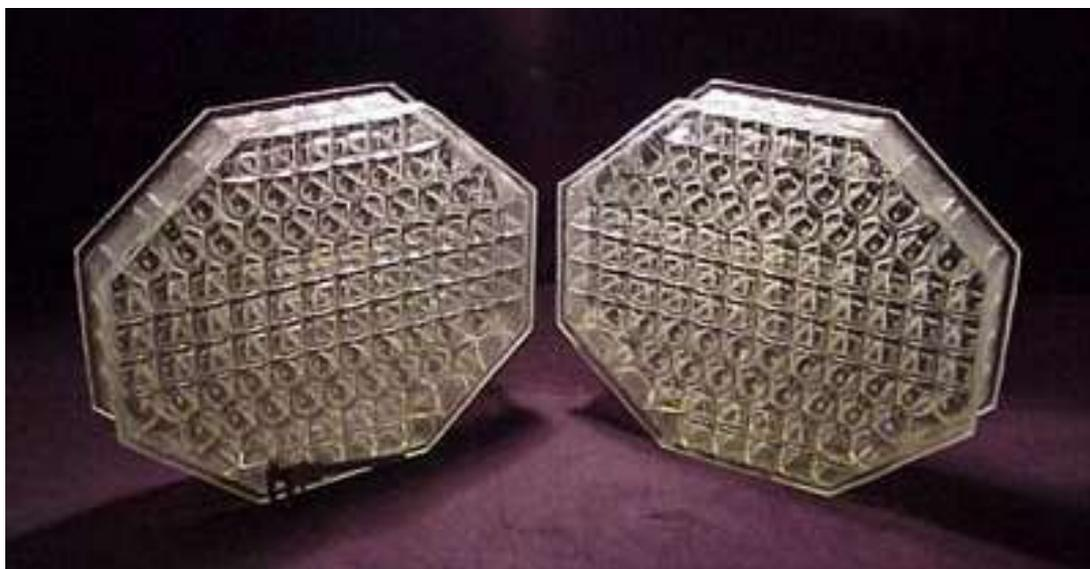
**Figure 38: Light-weighted Hextek borosilicate substrates as used for M3.**
