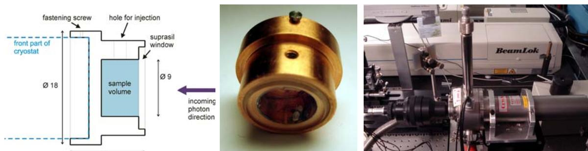
**Figure 3.** Axially symmetrical sketch of the custom-made cuvette for temperature dependent measurements (left). Setup for the temperature dependent Raman experiments on solution of  $[\text{Cu}_2\text{L}_2(\mu\text{-O})_2]\text{I}_2$  (center: picture of the cuvette, right: top view on the cryostat).
