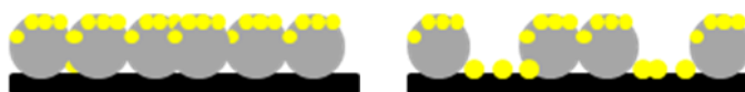
Figure 4.12 Sketch of the nanoparticle coverage for the case of hexagonally close-packed and randomly adsorbed dielectric spheres
