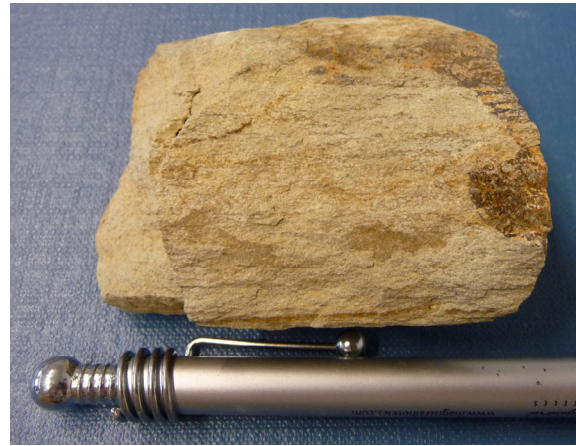
Fig. 2.4: Fine grained yellowish meta-sandstone of Neoproterozoic to Lower Cambrian metasedimentary units (#JU-21).
