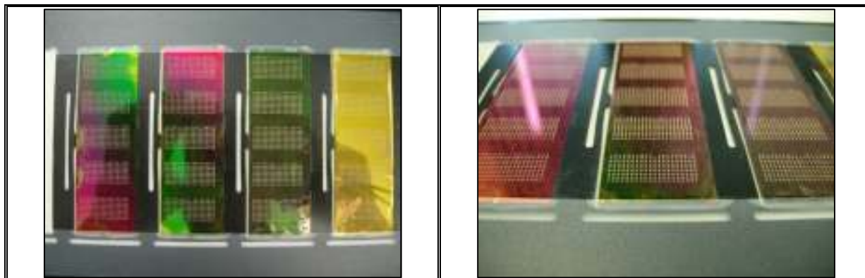
Figure 3-4. Polymer-coated LSPR biosensors after deposition of amino acids particles via a modified laser printer.
