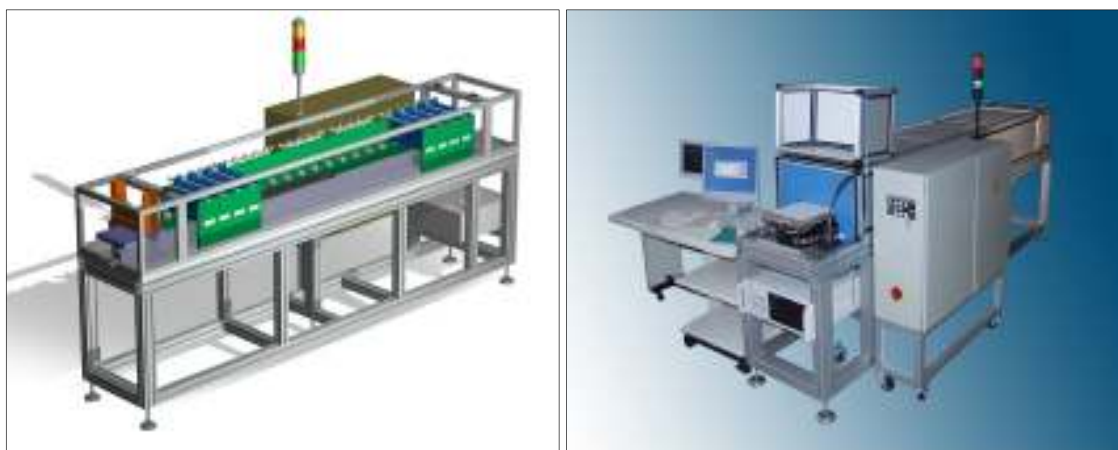
Figure 2-6. Peptide printer based on a color laser printer OKI C7400, equipped with 20 printing units, each containing one particular type of amino acid toner particles. 2
