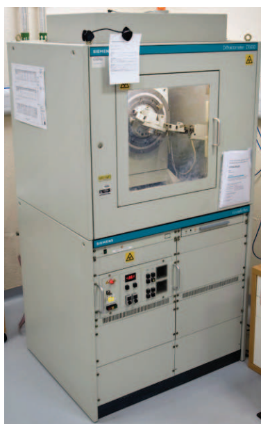
Fig. 2.3: Image of the X-ray diffractometer XRD D5000 from Bruker-AXS/Siemens (source: http://www.bruker-axs.com ).
