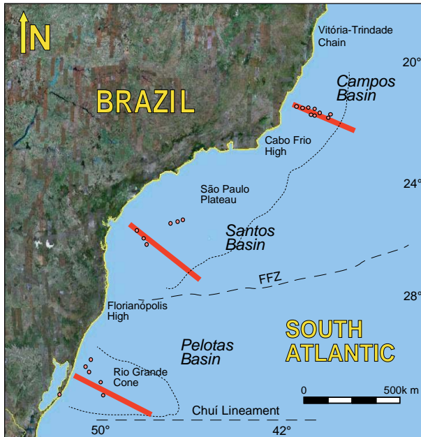
Fig. 3.1 Location of 2D seismic reflection profiles (red lines) and correlation wells (red points). Dashed lines represent the main structural-bathymetric provinces. FFZ: Florianópolis Fracture Zone.
