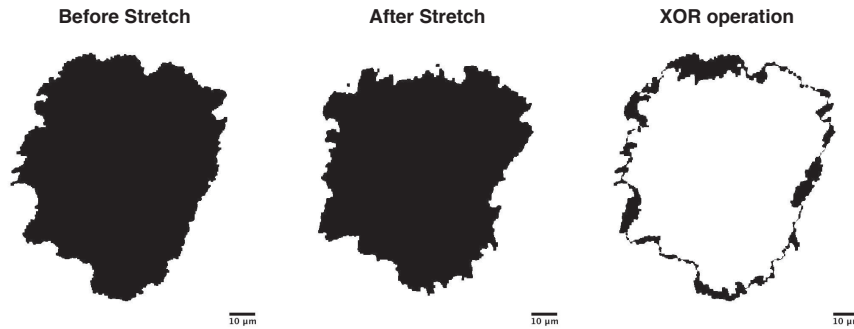
Figure 5.2: Visual description of the ImageJ iCalc macro. Using the XOR calculation between images embedded in ImageJ we can quantify protrusion activity.
