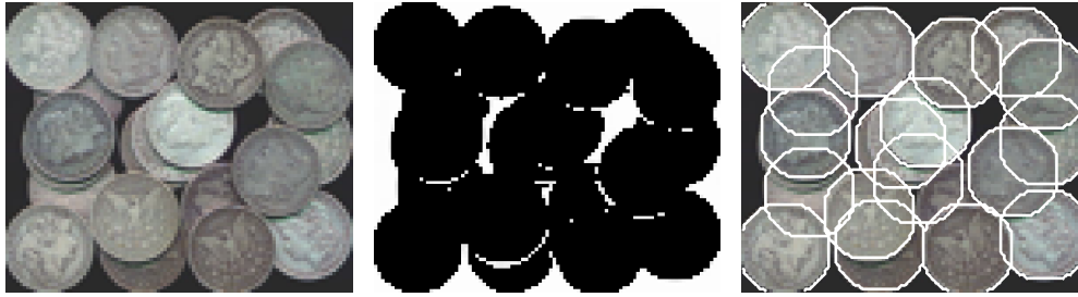
Figure 6.4. Application of the proposed approach to an image containing overlapping coins. Although not all objects are detected our approach reveals promising results and recognizes even highly occluded objects. Left: Input image. Center: Initial, local pre-segmentation obtained by inspecting the distance to the dark background color and local thresholding; used as input to the proposed method. Right: Final segmentation result of the proposed approach, computed solely from the pre-segmentation in the center. Although there are some mistakes, the method correctly detects most of the heavily-occluded objects on the lower levels.
