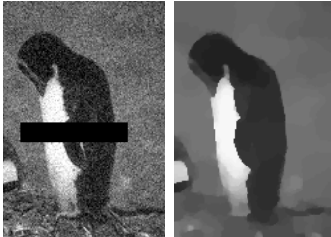
Figure 4.11. Denoising/inpainting problem with 64 classes and the nontrivial truncated linear metric. Left: Noisy input image with inpainting region marked black [SZS+06]; Right: Result of the DR method. The truncated linear metric d was approximated by an Euclidean embedding, which allows to handle problems with a large number of labels.
