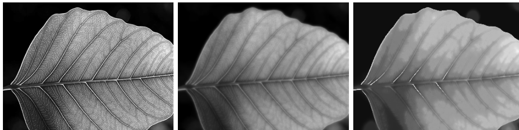
Figure 2.8. Approximation of the solution of the nonconvex Mumford-Shah problem using the “lifting” technique. Left: Input image. Center: Result of classical L^2 - L^2 denoising. Details are removed uniformly, which leads to loss of detail and smoothing at hard edges. Right: Result of variational denoising using the Mumford-Shah functional with 8 levels. Noise or fine details can be removed without blurring sharp edges. The lifting approach allows to approximately minimize the full Mumford-Shah functional by solving an associated labeling problem in a higher-dimensional space.
