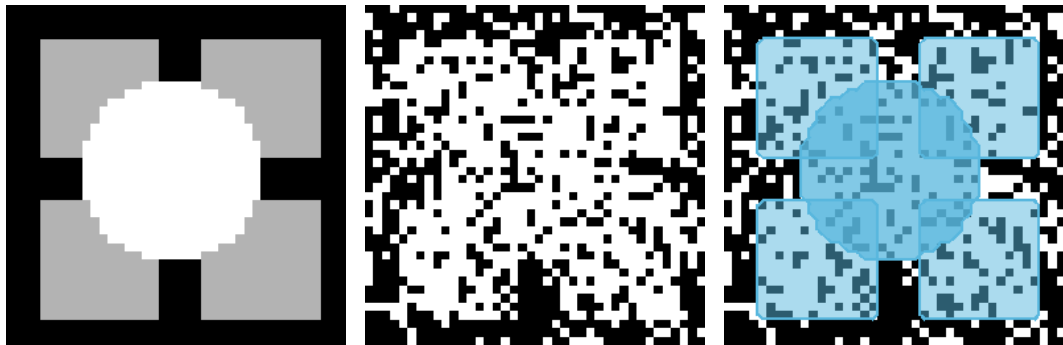
Figure 6.3. Synthetical example demonstrating the shape reconstruction capabilities of the proposed approach. Top left: Original image consisting of a circle and four squares. Top center: Local segmentation based on the gray value with heavy overlaid noise. This local pre-segmentation constitutes the input to the proposed method. Top right: Result obtained by our approach. The individual shapes are correctly identified with the aid of a dictionary of square and circular templates. In this case the output vector of the relaxed problem is integral, indicating that it is a minimizer of the original combinatorial problem, with each of the five nonzero entries corresponding to one of the five visible shape parts.
