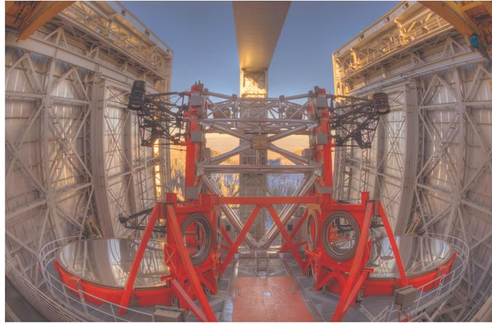
Figure 1.6: Picture of the LBT dome (courtesy of Marc-André Besel), taken 2008. One can identify the two primaries and the two prime focus cameras LBTC blue and red. The central focal station was not populated in 2008. Currently, LUCI I is installed in the front left bent focal station and LBTI in the central part. LINC-NIRVANA will go in the rear part (front in the picture).
