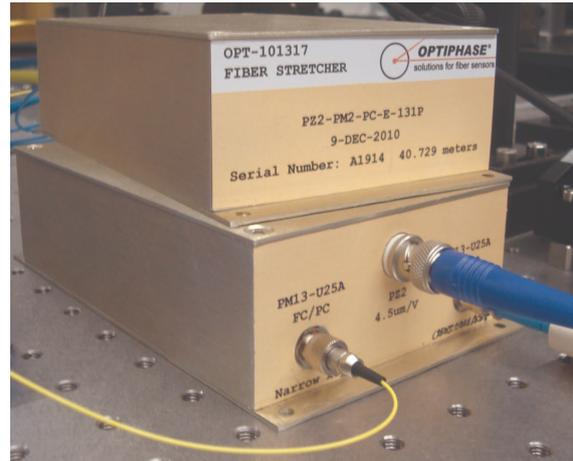
Figure 2.10: The two fiber stretcher devices. The inputs and output can be seen on the bottom device, while the other device is rotated by  $180^\circ$  for easier fiber cabling.
