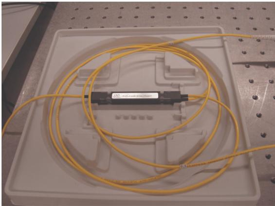
Figure 2.7: This Y-coupler splits the light injected at the fiber input on the left equally onto the two output ports on the right.
