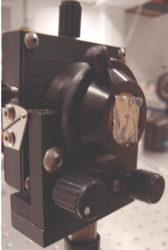
Figure 2.17: Front of the “blinking diode”. The pupil can be positioned in  $xy$ .
