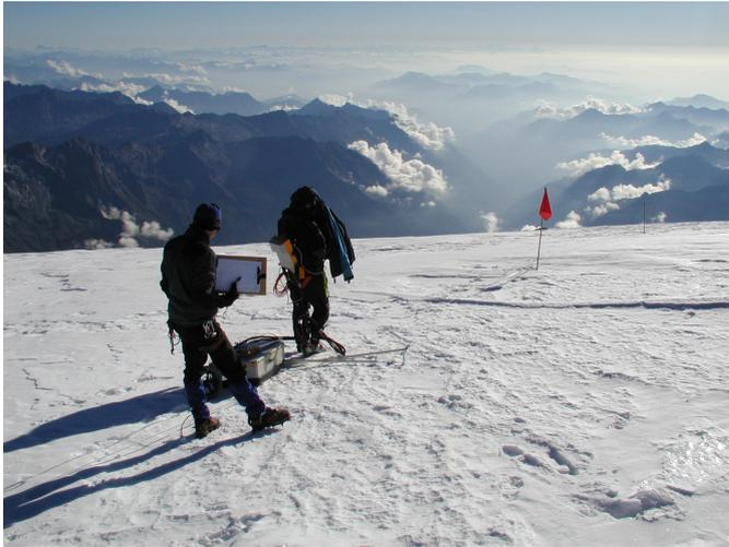
**Figure 3.4:** GPR common offset measurements at Colle Gnifetti. Transmitter and receiver are mounted on a sled pulled by hand. The transmitter is triggered by a distance wheel behind the sled. Picture from O.Eisen.
