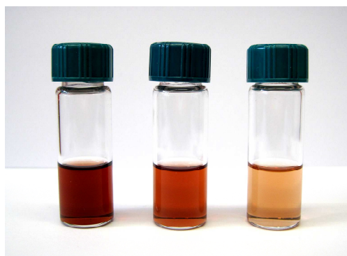
Figure 11 Selector-content of Chirasil-Vandyl-OC 3 visualized by dissolution of 42 , 43 and 44 in dichloromethane. Selector concentration (left to right): 20.0%, 10.2% and 3.5% V(O)(hfpc) 2 @PS.
