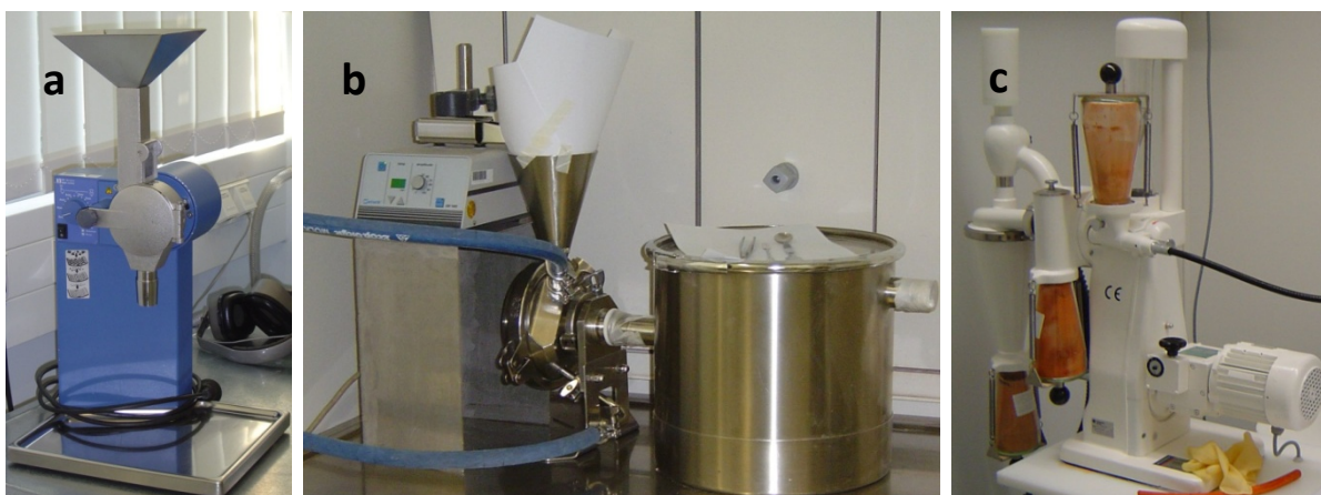
Figure 1.17: The blade granulator (a), the AS 100 air jet mill (b), and the winnower (c).
