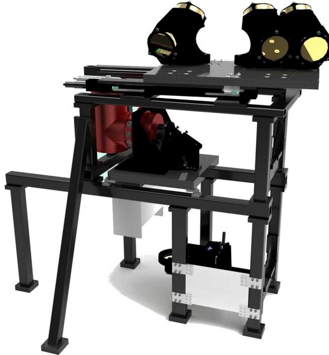
**Figure 4.4:** H+K-band NIR wavefront sensor that will be installed on all four 8-m UTs. Image credit: A.Huber and R.Rohloff.
