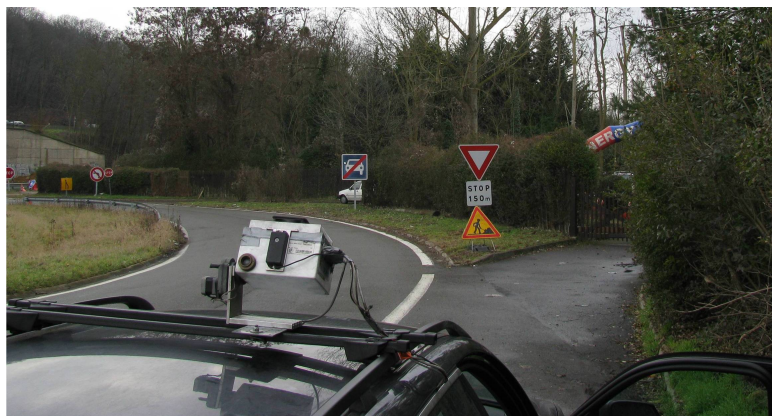
Figure 6.1: The mini MAX-DOAS instrument mounted on a car shown from different directions. The instrument is looking at 22^\circ elevation angle.
