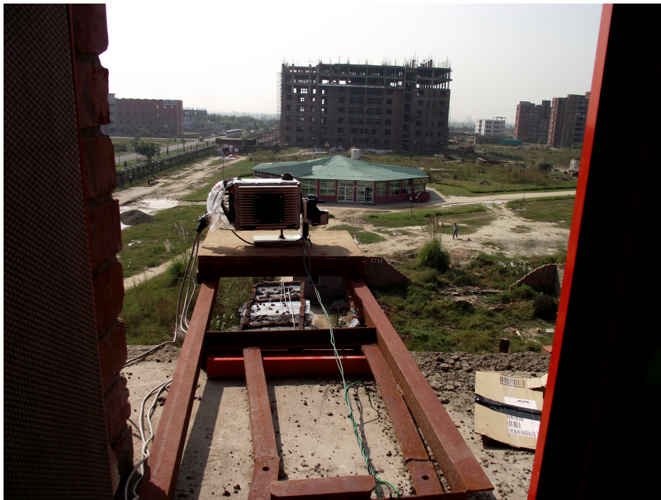
Figure 8.2: The mini MAX-DOAS instrument mounted at a window side at Sharda university in Greater Noida.
