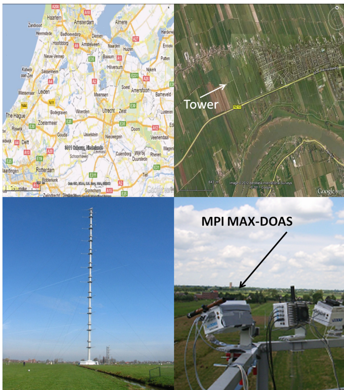
Figure 7.1: Left (top): the Cabauw site is located near Lopik in The Netherlands, in SW of Utrecht. Right (top): The Cabauw meteorological site has a tower, where the MPI instrument was located. Left (down): The Tower. Right (down): MPI mini MAX-DOAS with other mini MAX-DOAS instruments from BIRA and KNMI.
