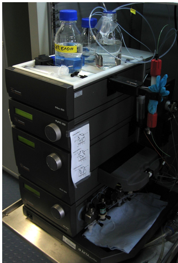
Figure 8.1: Photograph of the ÄKTA purifier system equipped with a heparin column. The setup contains a pump to apply sample and buffer to the column and various analytical instruments like spectrophotometer to monitor absorption or pH-meter to measure the pH.
