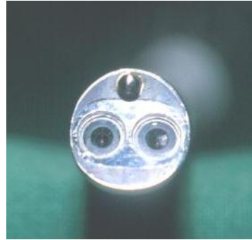
Fig. 5.12: Top: Distal end of 3D thoracoscope with two objective lenses and irrigation canal. Left: Head mounted liquid crystal display (LCD) for endoscopic operations (1). The microphone (2) can be used to load any type of image, i.e. x-rays, and CT or MRI images.
