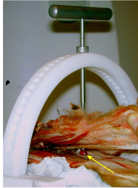
Fig. 7.5: Evaluation of the puncture algorithm and precision of the puncture device using a Gd pallet (arrow). The sheep thigh bone was cut in half so that easy positioning of the pallet could be achieved.
