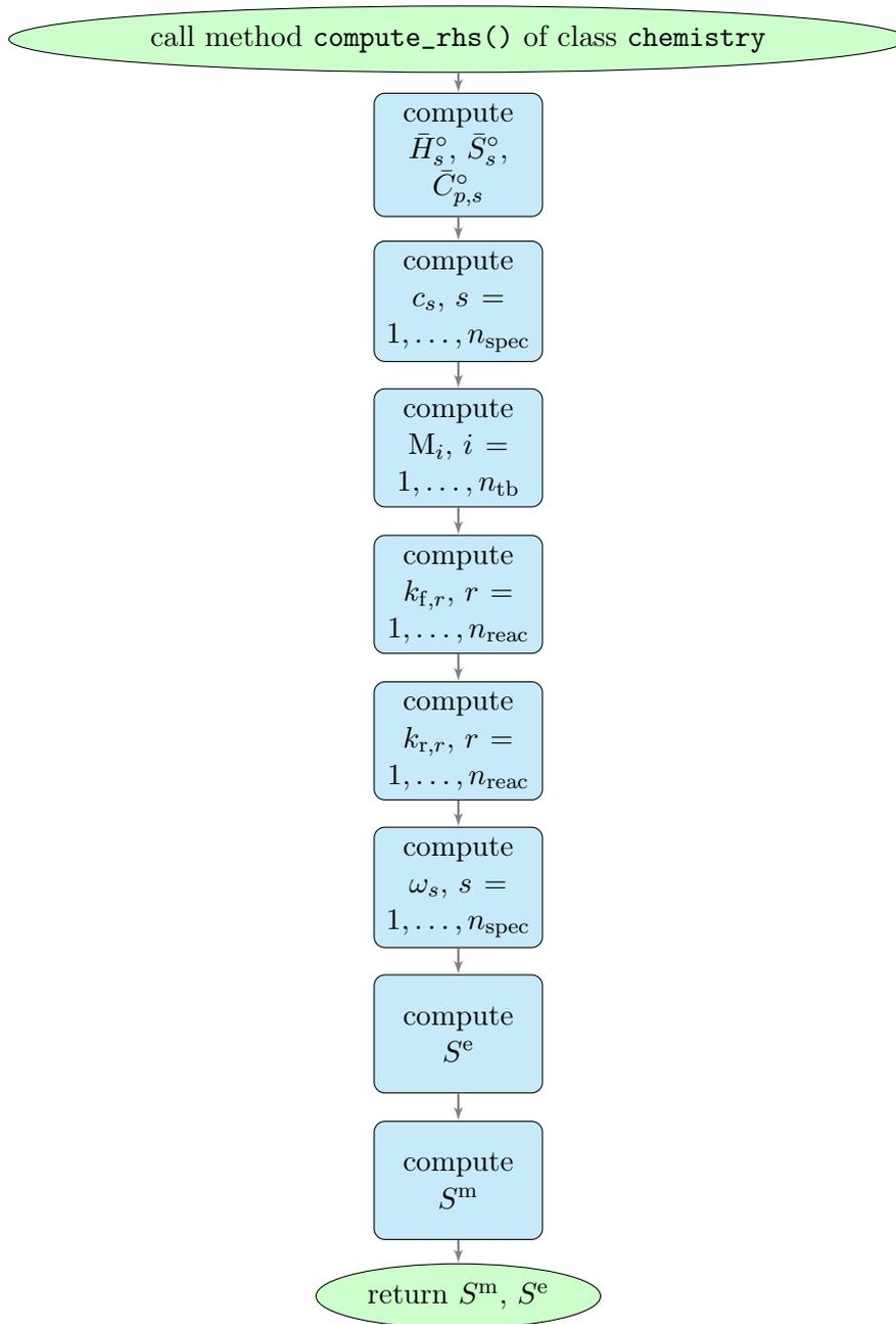
**Figure D.2:** Flowchart of the computation of the right hand side of the ODE of the combustion model in the model reduction code MoRe.
