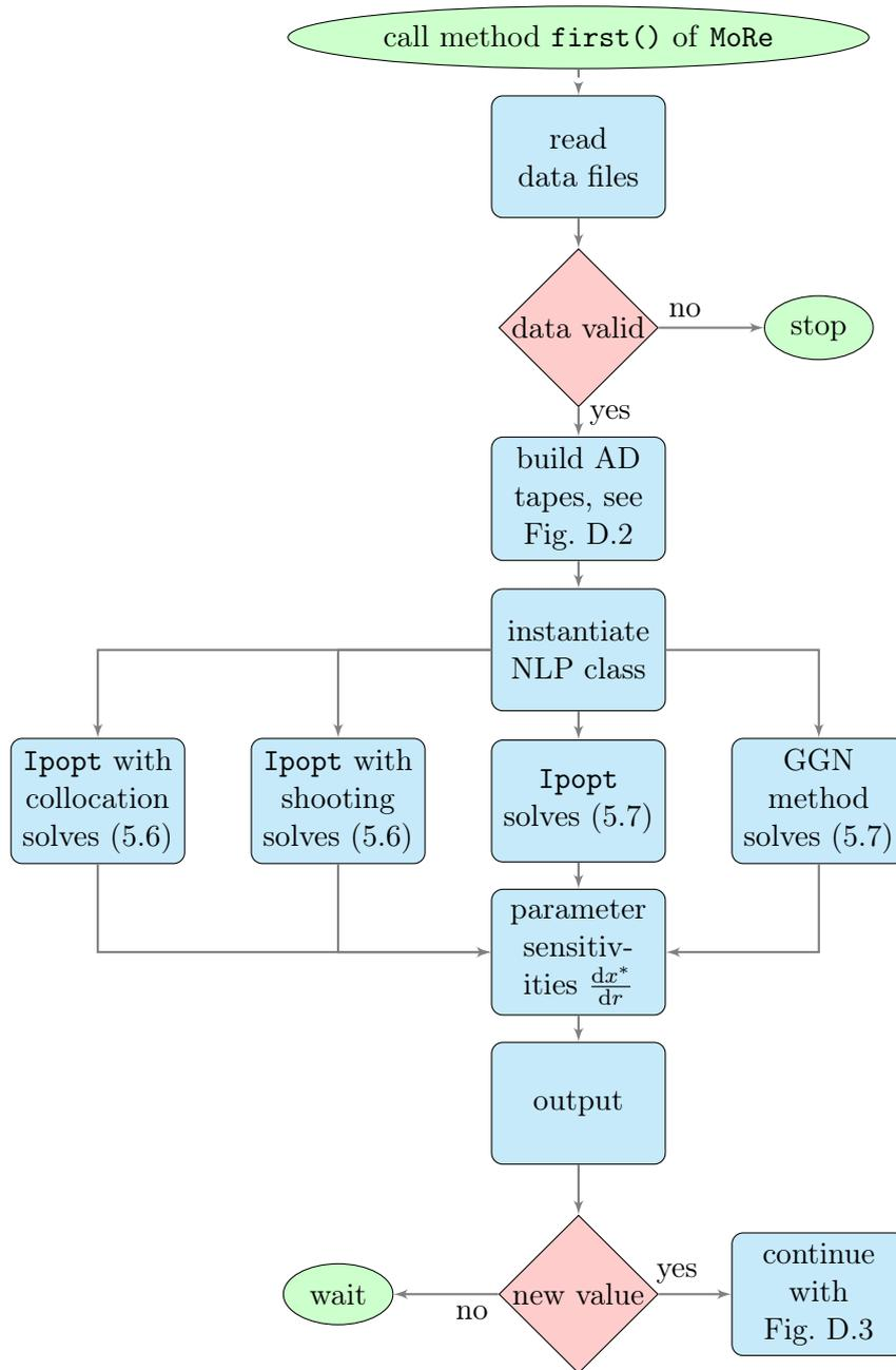
**Figure D.1:** Flowchart of a first call of the model reduction code MoRe with method `first()` or `reduction()`.
