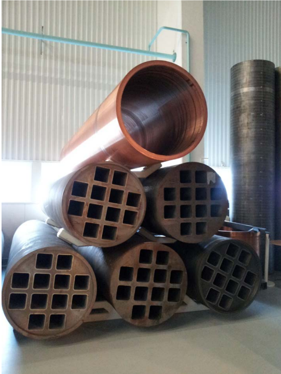
Figure 2.1-1: Various parts of the canister: steel cylindrical structures, with cavities for the allocation of fuel assemblies, and the copper outer body (at the SKB Canister Laboratory in Oskarshamn, Sweden).
