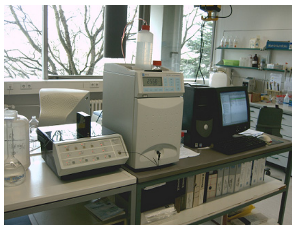
Fig. IV.1: Ion chromatography station comprising automatic sampler, ion chromatograph and computer. The chromatograph consists of a pump, an injection valve with a sample loop (a), a self-regenerating suppressor (b), a guard column (c), an anion-exchange column (d) and a conductivity cell (e).
