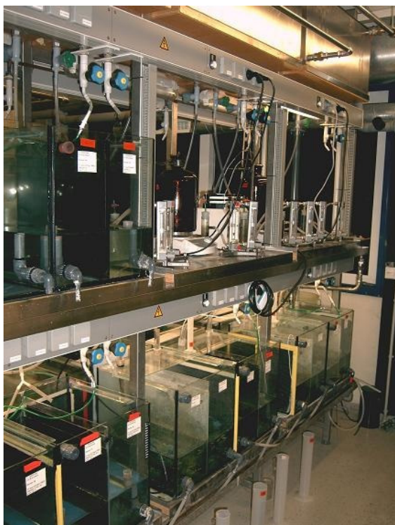
Fig. III.1: Flow through system comprehending tap water storage tanks, particle depositors and rotameters for water flow as well as MMS stock solutions (green) and pumps. In addition, tanks are aerated and heated. Cylinders are used for daily calibration of water and stock solution flow.
