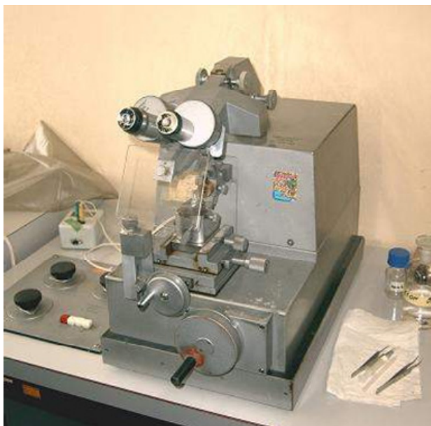
Fig. II.2: Ultramicrotome used for preparation of semithin sections of liver, gill and gonad samples embedded in Spurr's resin.
