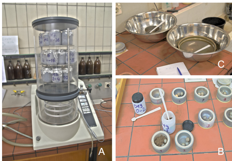
Fig.13 A) The small freeze-drying unit Steris Lyovac GT2. B) The freeze-dried samples are placed into agate cups, which are used for the planetary ball mill Fritsch Pulverisette GT2. C) Subsequently, all samples are sieved again (100 mesh) to remove the remaining small organic components.
