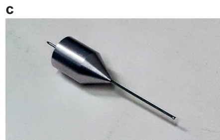
Fig. 3.3: Coating in the ZEISS Merlin. (a) Evaporator head with cylindrical aperture tube attached. Cover shield not shown. (b) Evaporator in operation inside the ZEISS Merlin. (c) Pointing tool for visual aiming.
