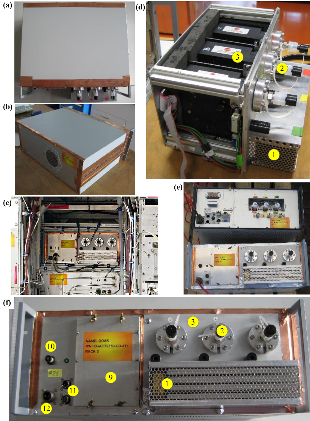
Figure 6.5.: Photographs of the DOAS container instrument, cf. Table 6.1 concerning the depicted numbers. (a) top side (b) back side with blowhole for ventilator, edging taped with EMC tape (c) installed in the CARIBIC Container (cf. Fig. 5.4) (d) opened spectrograph box (e) old and new instrument (f) front side
