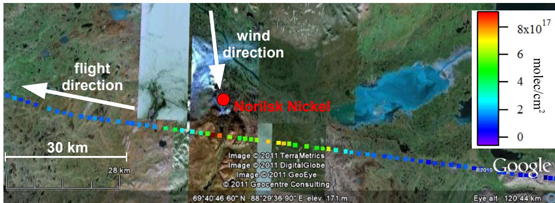
Figure 7.21.: Flight path close to Norilsk, color-coded with \text{SO}_2 SCD for the nadir direction. The section depicts the flight route between 07:10 UTC (right image border) and 07:20 UTC (left border). The closest distance to Norilsk was at 07:15 UTC, where the highest \text{SO}_2 SCD were observed.
