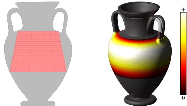
Figure 3: Heat map visualization of the distance to a fitted cone. Due to the high curvature of the vessel (KHM Inv.-No. 3601) larger distances at the middle part of the frustum are visible.
