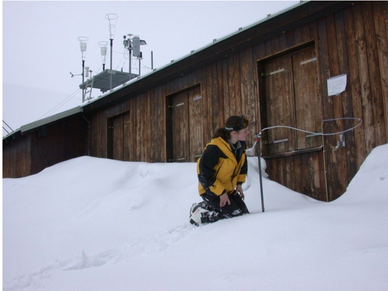
Fig. 4-8 Sampling of atmospheric mercury at the limnological station of the University of Innsbruck at Lake Gossenkölle. In front: Inlet for TGM; on the roof: measurement of meteorological data and precipitation sampling.
