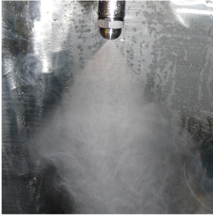
Fig. 4.1: Photograph of the water spray formation.
