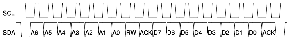
Figure 3.3: I 2 C Transmission — SCL: Clock signal — SDA: Data signal.
