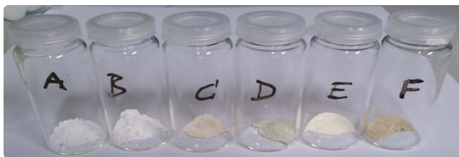
Figure 3.8: TiO 2 nanoparticles: A) EVONIK P25 B) “B1” similar to P25 with smaller particle size. With metal impregnation in weight %: C) 0.1 % Pd D) 0.5 % Cu E) 0.1 % Pt F) 1 % Pt.
