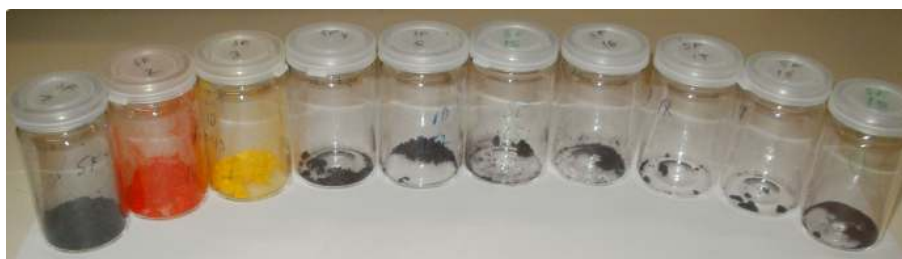
Figure 3.9: Powder samples of the provided dyes (from left to right SF1-SF5 and SF15-SF18). The structural formulas can be found in Figure 3.10.
