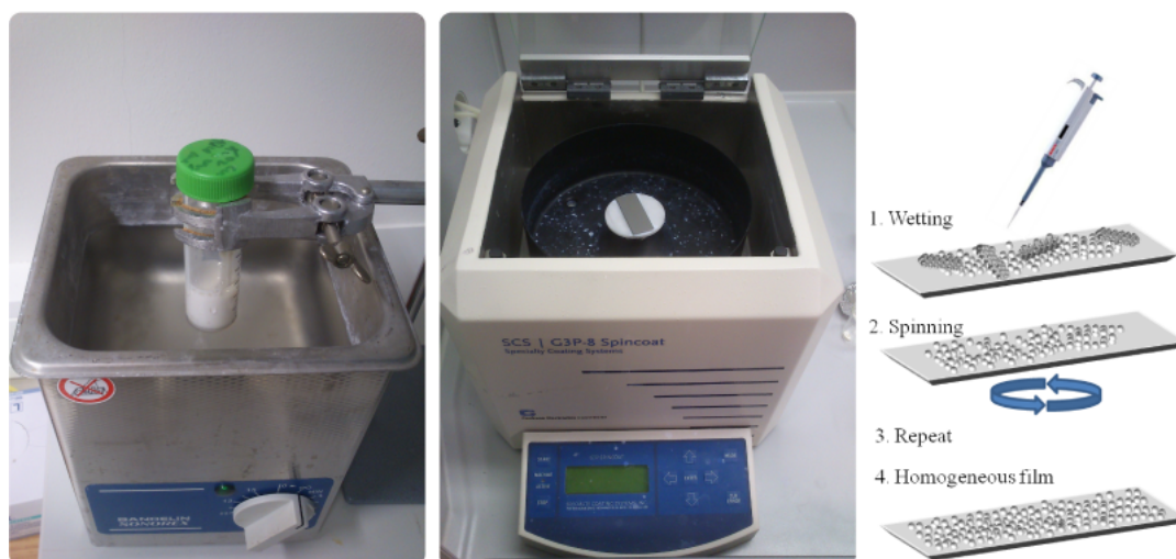
Figure 3.11: Preparation methods for thin film preparation: Ultra sonic bath (left), spin coater with substrate (middle) and preparation routine (right). A fast spin coating reduces the attachment of particle agglomerations. With multiple spin cycles a closed, homogenous film is achieved.
