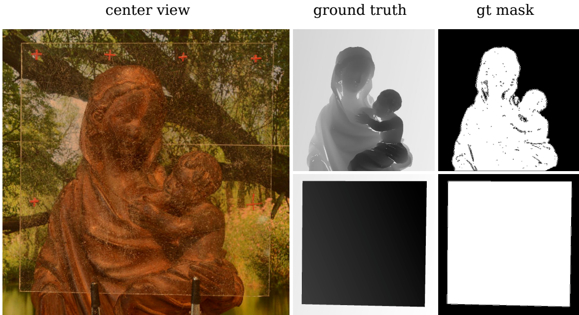
Figure 20: Data set transparency . Left: center view, middle top: depth of the background, middle bottom: depth of the foreground, right top: background mask for valid depth ground truth pixel, right bottom: foreground mask for valid depth ground truth pixel.
