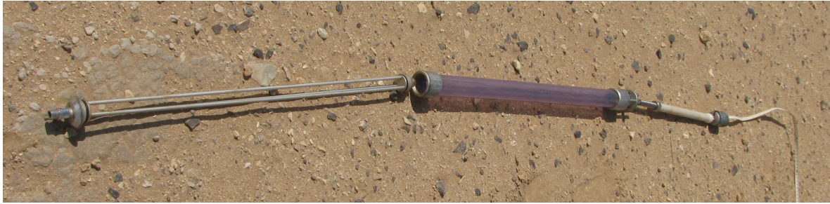
Figure 5.2: The deep sampler used to get water samples from open borehole without a pump. It is depicted in its open state. A weight is sent down along the cable enables to close the sampler at the desired depth.
