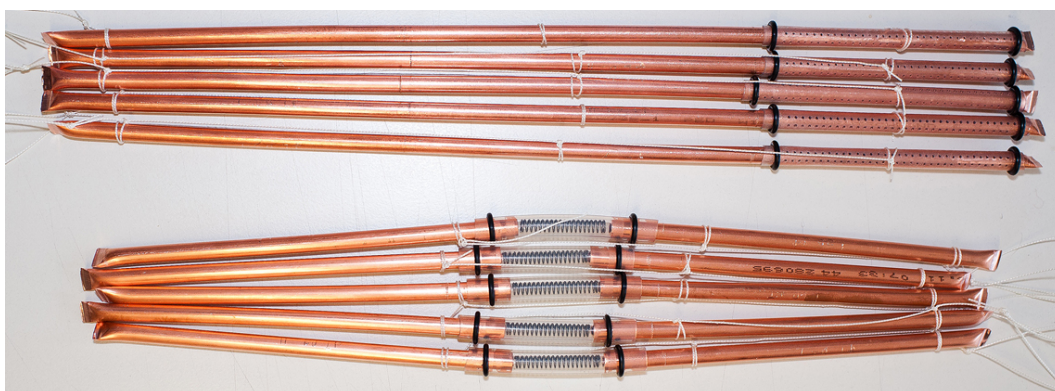
Figure 5.1: Two sets of diffusion samplers used in this study. The lower ones are the normal diffusion samplers, consisting of two separate copper tubes connected by a PVC tube. The upper version of diffusion samplers was constructed to withstand the high hydrostatic pressure in the deep boreholes.
