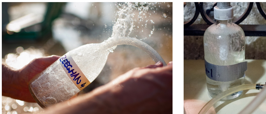
Figure A.12: Heavy degassing occurred during sampling and foam formation at the radon measurement of the Zeeghan wells
