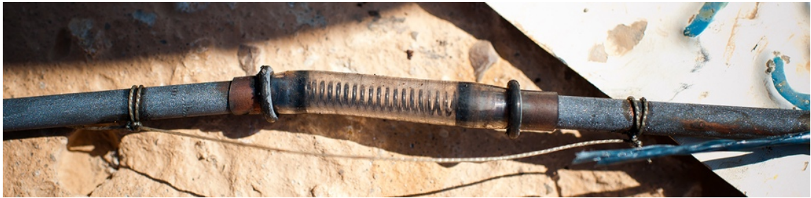
(c) The 569 m diffusion sampler was inflated after being retrieved to the surface.
