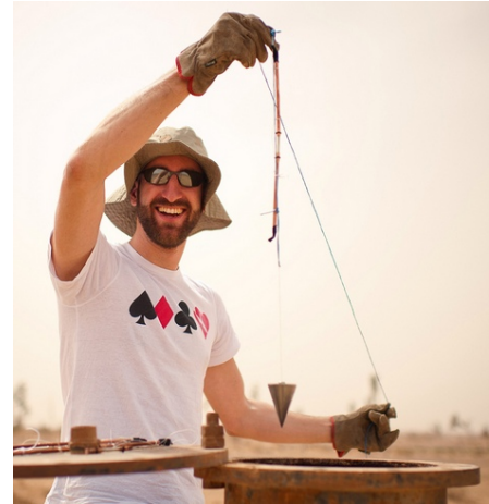
(b) Lowering the deepest diffusion sampler, an additional weight is attached.
