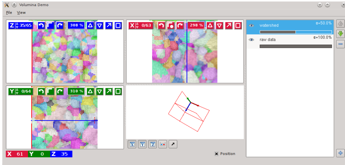
Figure 3.3: The VOLUMINA viewer shows a 3D dataset with a watershed segmentation overlay. The code to bring up this view is printed in Listing 3.1.
