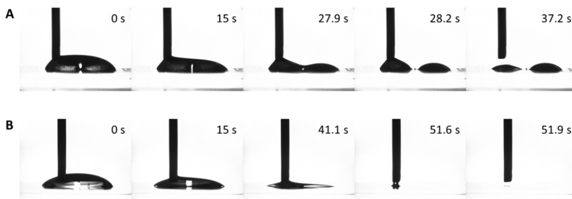
Fig. 5.2. A. Withdrawing of the water droplet from two coalesced 3×3 mm hydrophilic spots separated by 500 μm superhydrophobic barrier ( \theta_{\text{adv}} = 167^\circ ). B. Withdrawing of the water droplets from two coalesced 3×3 mm hydrophilic spots separated by 500 μm highly hydrophobic barrier ( \theta_{\text{adv}} = 128^\circ ).
