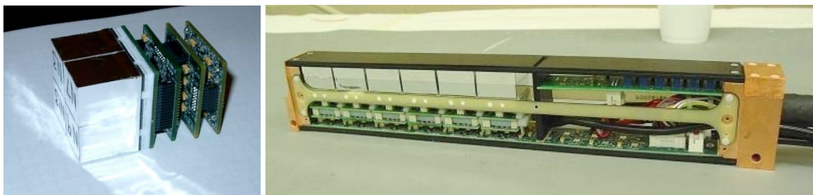
Figure 4.9 Photographs of the module (left) and module assembly (right) used by Siemens in the BrainPET. From [67].
